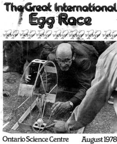
FIGURE 7.1. The poster for the eggmobile contest. In 1978, the Ontario Science Centre in Toronto sponsored a contest to see how far an egg could be propelled using a single rubber band for power. The idea was to design a very energy efficient transportation system. Ian Howard won the Canadian championship with the eggmobile shown here. In the international competition Ian moved the egg 351.21 meters and placed a close second behind Steve Darling, a Rolls-Royce engineer.
